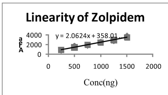
Fig.4: Linearity curve of ZOL at 254 nm
