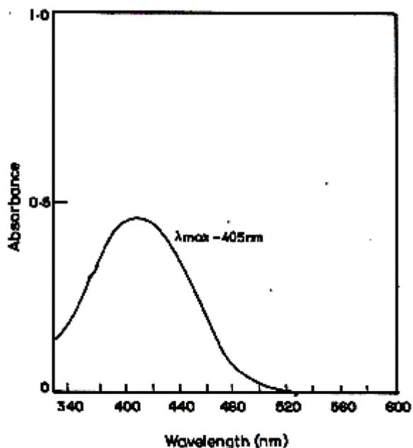
Fig. 3: Absorption maxima of nicorandil by colorimetry
