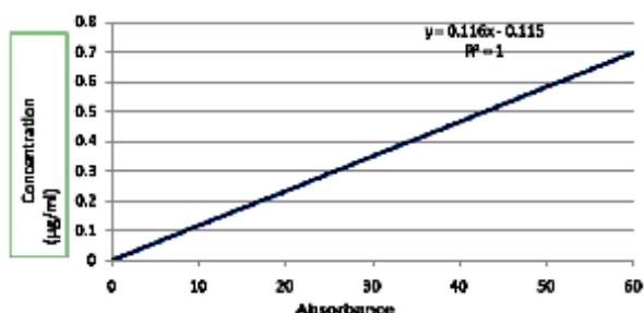
Fig.4: Standard calibration plot of nicorandil by colorimetry
